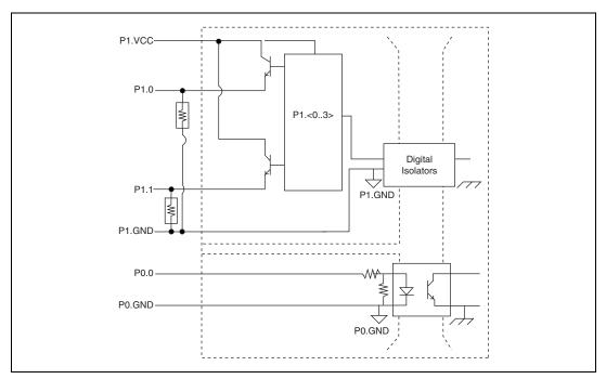
Figure 6-1. NI 6232 Digital I/O Connections (DO Source)
